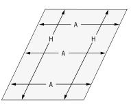
Measure at several points in case of possible frame size tolerances.
