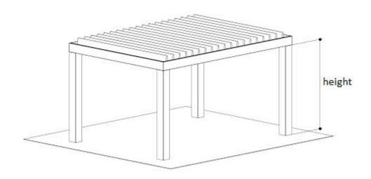
DURING MEASUREMENT, IT IS NECESSARY TO DETERMINE OTHER OPTIONAL ACCESSORIES SUCH AS LIGHTING, RAIN SENSOR, ETC. THEN IS APPROPRIATE TIME TO SPECIFY CONSTRUCTION FOR FOLLOWING INSTALLATION OF THE ENTIRE PERGOLA SYSTEM (ANCHORAGES, WATER DRAINAGE, ENGINE LOCATION, ELECTRICAL LINES, ETC.)
