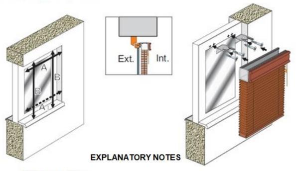
WIDTH = A - 2 cm A1= blinds width check (if A1 is smaller than A, A1 is the overriding width)
