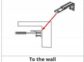
Fastenings will not be included in the delivery. In this case, it is not possible to predict the type of material you will be anchoring to. The mounting kit will include only mounting clips or brackets.
