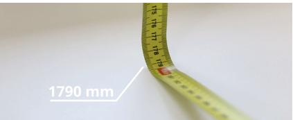
**Example of measurement:** The measured height of the blind, including the upper profile on the windowsill, is 1,800 mm, you can subtract -10 mm to -30 mm from the parameters (recommended subtraction for the height to the windowsill). For our example, we chose the subtraction -20 mm, **height = 1,780 mm**. You enter the values in bold in the order form.
