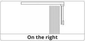
The control side cord&chain is chosen from the room towards the blind. The standard length of the control is 2/3 of the height of the blind.
