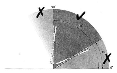
ATTENTION!!! THE ANGLE OF THE ROOFDECLINATION MUST NOT BE LESS THAN 30° AND MORE THAN 90°.
